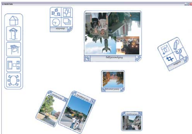
Figure 13: The DoHM client as it looks when supporting collaborative picture sorting. The icons on the left are PlaceRep icons for surfaces in the home. The floating toolbars contain tools for interaction with objects.
