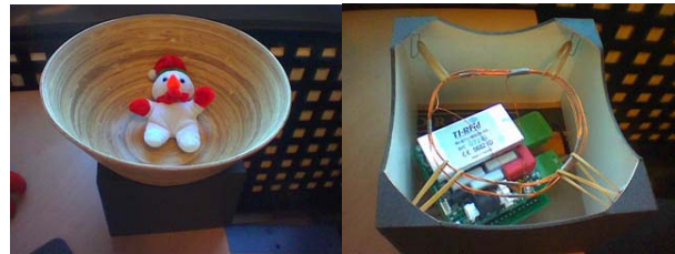
Figure 14: MediaTray for physical hypermedia interaction. The right picture shows the RFID tagreader in the bottom.
