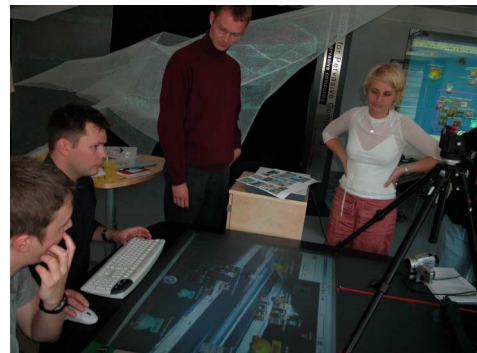
Figure 7: Interactive desk with tag-reader and snap-scanner as implemented in the initial test environment.
